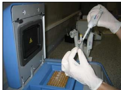
Grinding leaf samples with a tissue homogenizer
